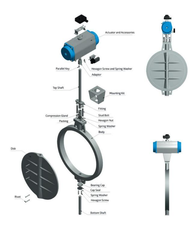
Exploded view of a standard GD-6 with a swing through cast-iron disk and a pneumatic actuator.
