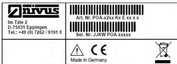
Fig. 4-39 Nameplate sensor POA
